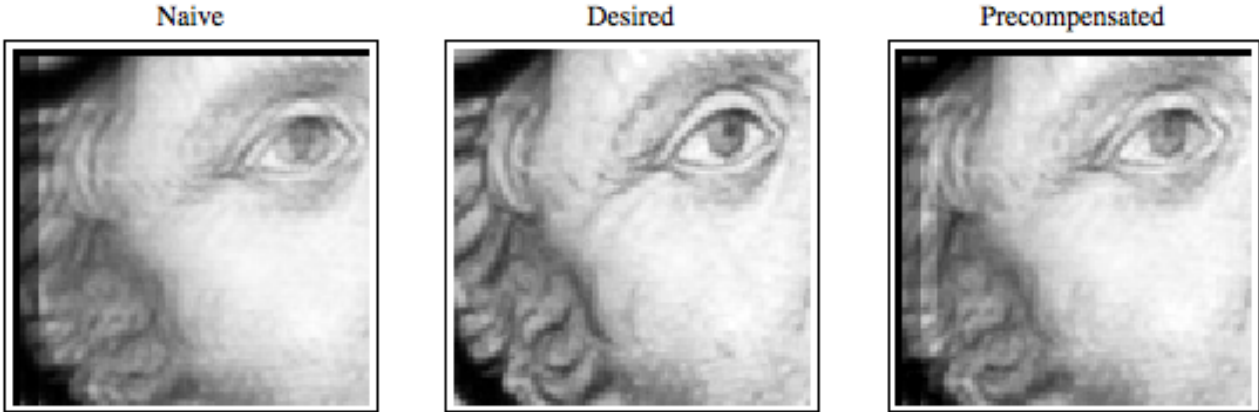
Figure 12: Comparison of precompensated image for a 2-D display with a pixel replication artifact.
